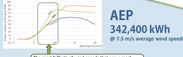
The most "effective" wind speeds that occur **most frequently** are 6 - 11 m/s. ZECWP 75kW turbine has the **highest energy production** at these wind speeds.
