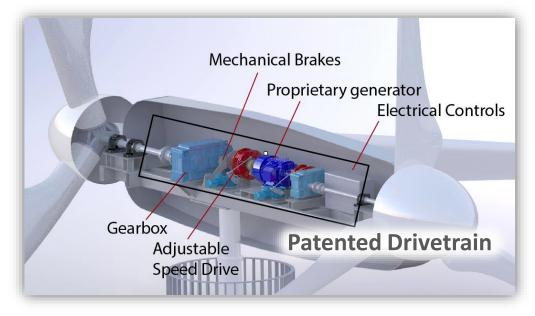
Our innovative drivetrain design is optimized for maximum energy production at all frequent wind speeds. System safety and reliability is our top priority.
